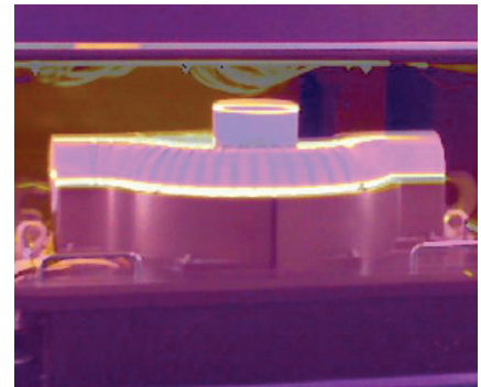
As part of the quality control process, Nexeo Plastics recommended adding thermal imaging to inspect the weld along the entire seam of the vent and ensure a water-tight fit.
